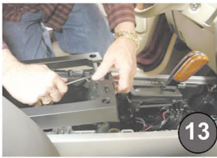
Gently pry up upper glove box housing and set aside.
