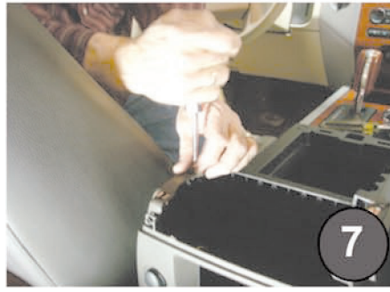
Remove 7mm screws on top of console.
