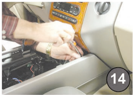
Remove 7mm screws (two in front and two in back)
