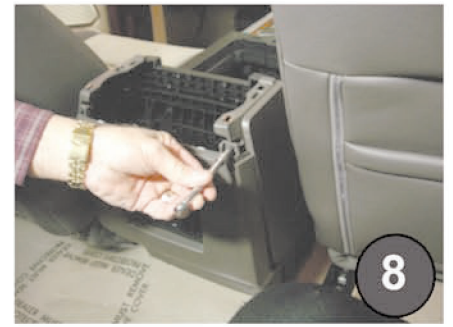
Use 7/32" socket to remove (2) rear screws.
