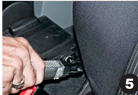
5 Remove 10mm bolts at the rear of the OEM floor plate. One per side.
