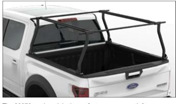
The 30070 truck rack is the perfect crossover rack for your adventures both on and off the job. Built to withstand the rigors of the workplace or a rigorous trip to your favorite kayak run. Load up with materials or all the gear for your next excursion. This rack features sturdy 2" steel pillars and 1.25" cross bars 0
